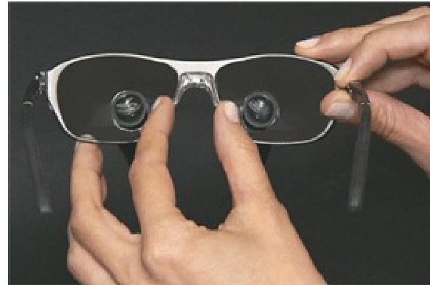
Loupes fits too low: tighten the nose pad to adjust the fitting
